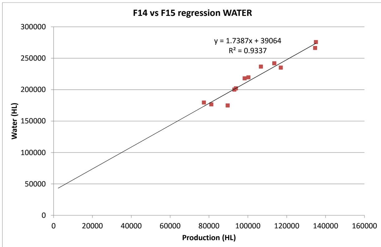
Figure 1. Regression analyses of production and water consumption.
